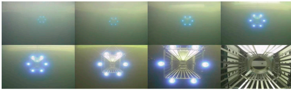
FIGURE 7 Docking process image in water pool.
