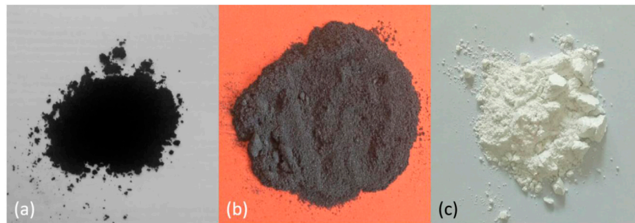
FIGURE 1 (A) Carbon black NPs, (B) graphene nanoplatelets, and (C) MgO nanoparticles.
