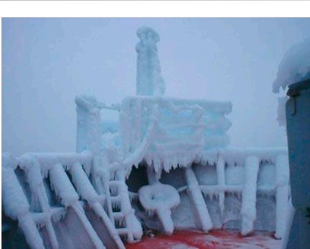
FIGURE 2 Superstructure icing (Mahmood and Revenga, 2006).
