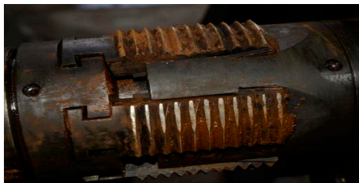
FIGURE 14 | Wear condition of No. 1 slip group.
