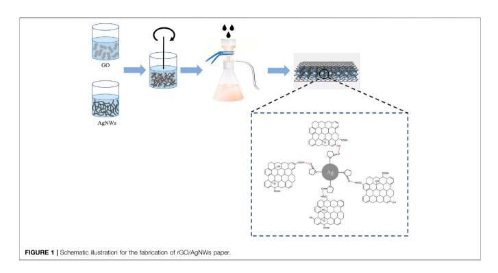
EG) were added to the mixture, then immediately placed into a reactor and allowed to stand at 160°C for 3 h. Finally, the solid was consecutively washed with ethanol and acetone by centrifugation of 4500 rpm for 7 min to remove the excess chemicals and the silver nanoparticles (AgNPs). The obtained AgNWs were diluted with ethanol to a concentration of 0.4 mg/ml before use.
