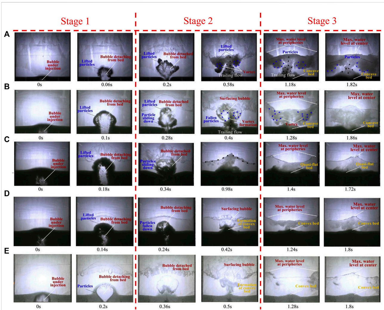
FIGURE 10 Typical sloshing motion under gas-injection conditions with solid particles (spherical glass particles, \Delta T = 0.1 s) (Cheng et al., 2019b). (A) Regime I ( d_p = 0.125 mm, H_{pb} = 15 cm, p = 3 bar). (B) Regime II ( d_p = 0.5 mm, H_{pb} = 15 cm, p = 3 bar). (C) Regime II ( d_p = 0.5 mm, H_{pb} = 30 cm, p = 3 bar). (D) Regime II ( d_p = 0.5 mm, H_{pb} = 30 cm, p = 2 bar). (E) Regime III ( d_p = 6 mm, H_{pb} = 15 cm, p = 3 bar).
