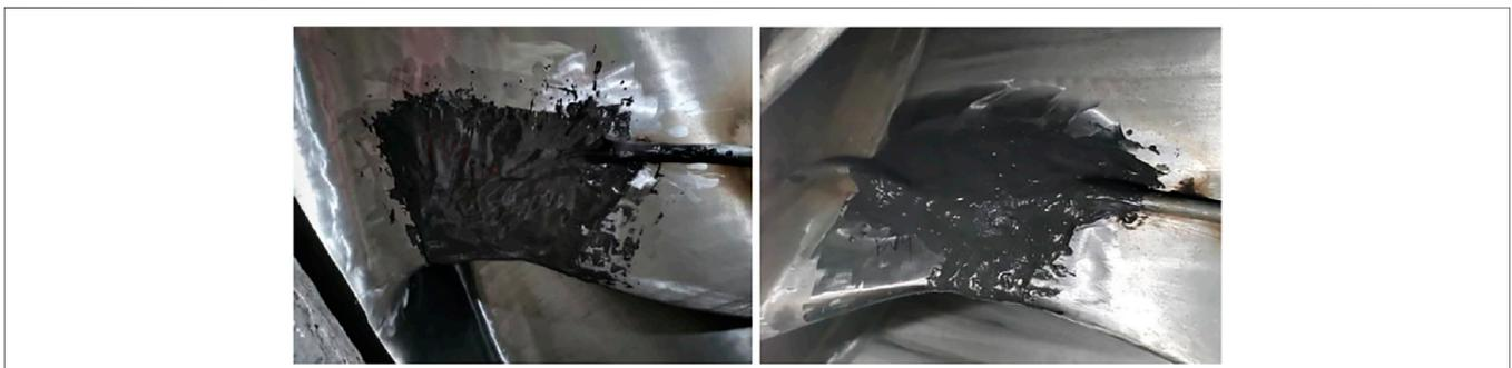
**FIGURE 6** | The photos of protection of the strain gauges by metal protective coating.
