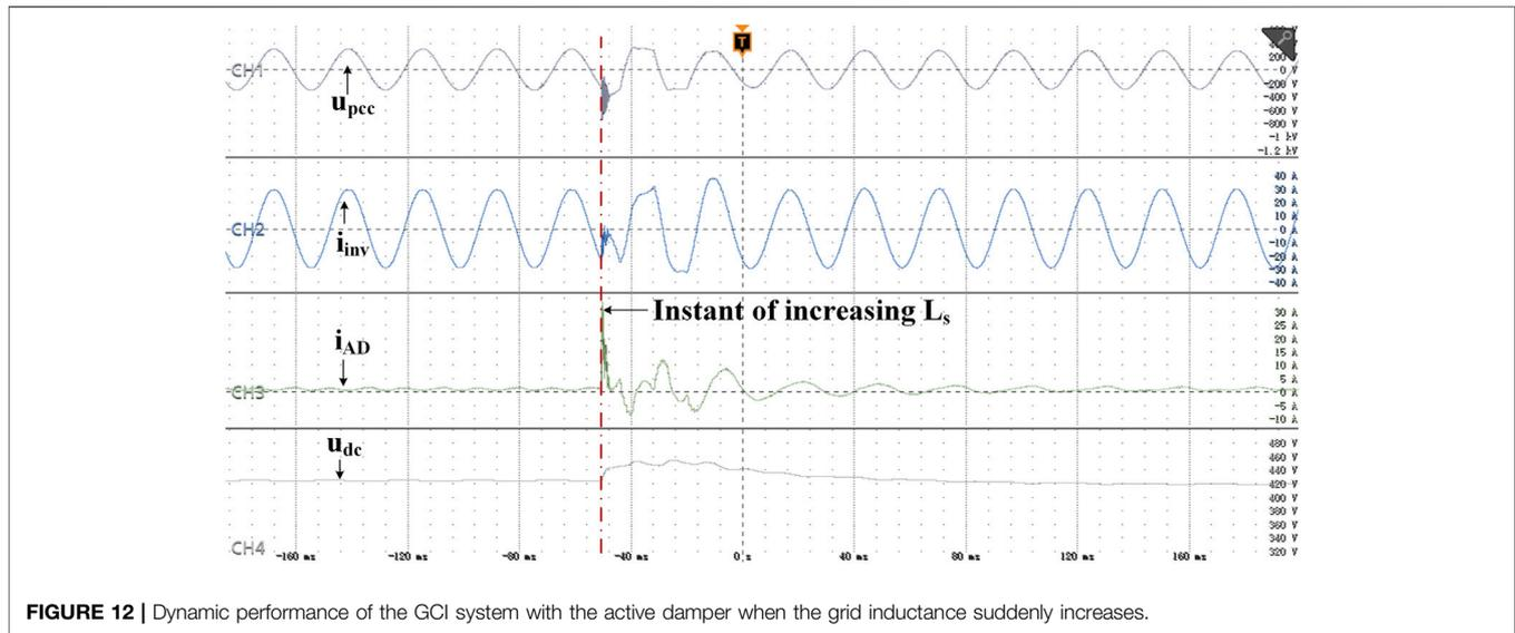
**FIGURE 12** | Dynamic performance of the GCI system with the active damper when the grid inductance suddenly increases.
