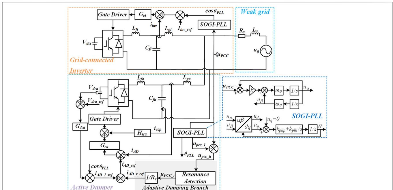
**FIGURE 1** | Grid-connected inverter system with the active damper under weak grid.
