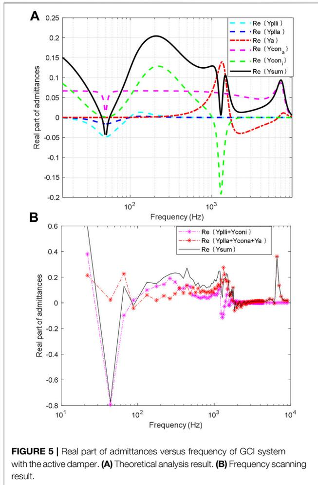
**FIGURE 5 |** Real part of admittances versus frequency of GCI system with the active damper. (A) Theoretical analysis result. (B) Frequency scanning result.
