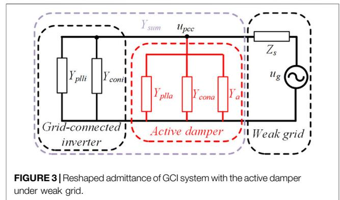
**FIGURE 3** | Reshaped admittance of GCI system with the active damper under weak grid.
