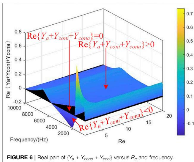
**FIGURE 6 |** Real part of  $\{Y_a + Y_{con_a} + Y_{con_i}\}$  versus  $R_e$  and frequency.
