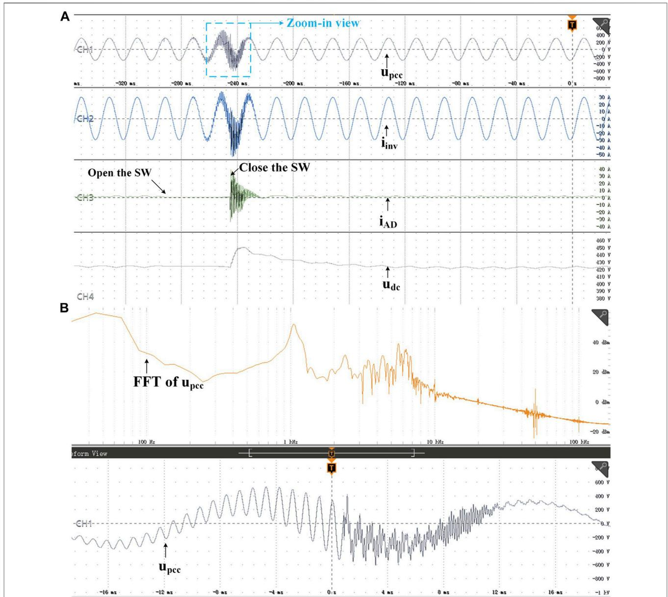
**FIGURE 9 |** Dynamic performance of plugging in and removing the active damper by opening and closing the switch. **(A)** Overall view. **(B)** Zoom-in view and corresponding FFT analysis.
