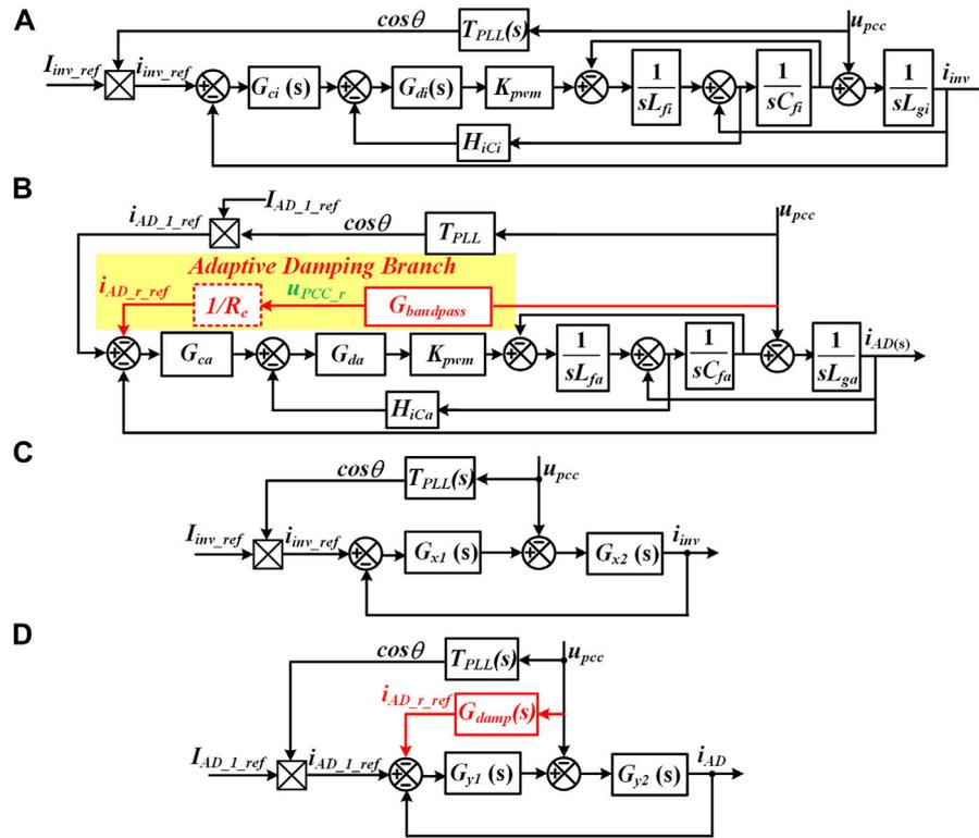
**FIGURE 2** | Mathematical models of the GCI and active damper and corresponding simplified models. **(A)** Mathematical model of the GCI. **(B)** Mathematical model of the active damper. **(C)** Simplified model of the GCI. **(D)** Simplified model of the active damper.
