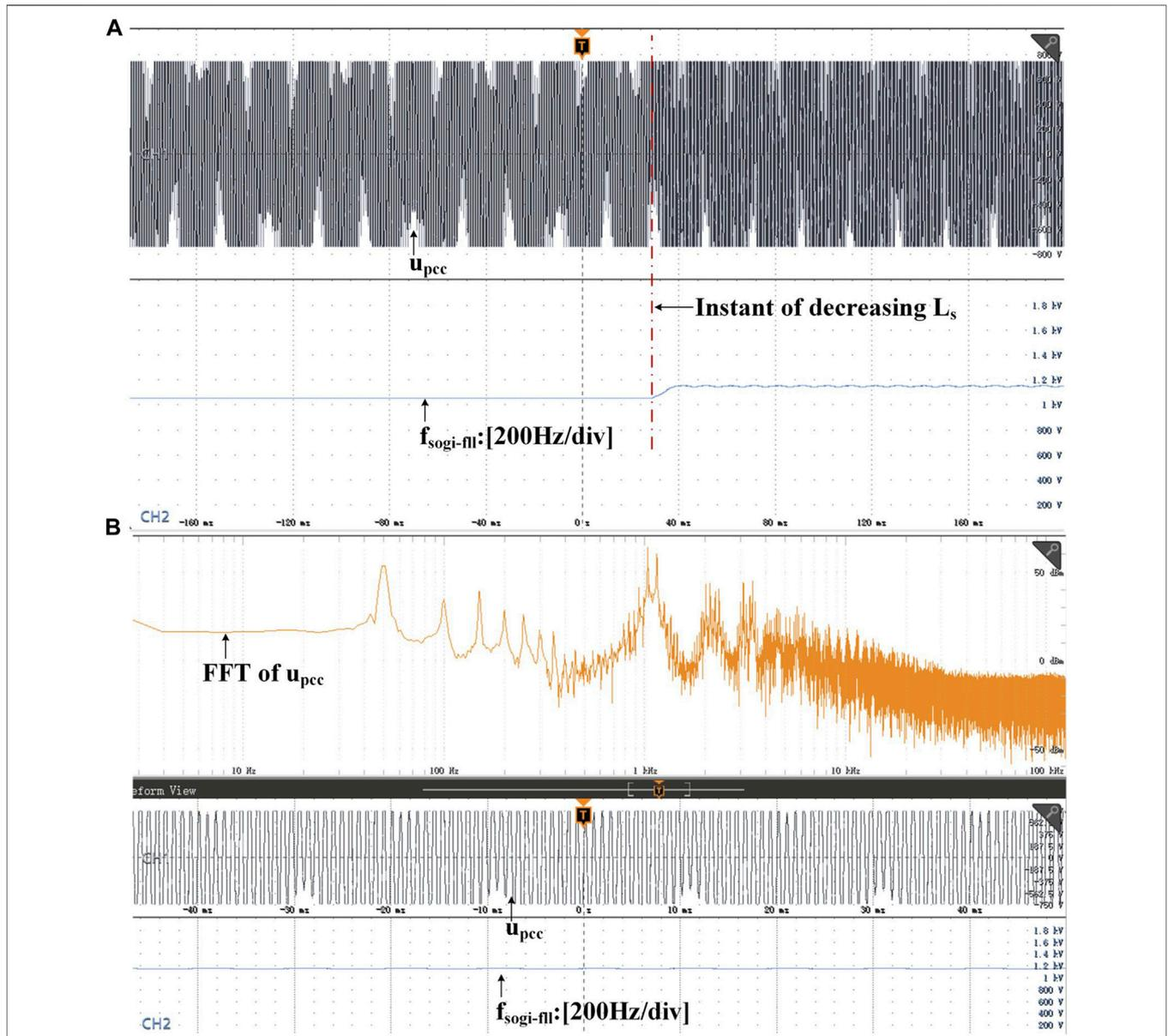
**FIGURE 10 |** Resonance detection of the SOGI-FLL. **(A)** Dynamic waveform when  $L_s$  decreases. **(B)** FFT analysis and resonance frequency detection result of the  $u_{pcc}$  in steady-state.
