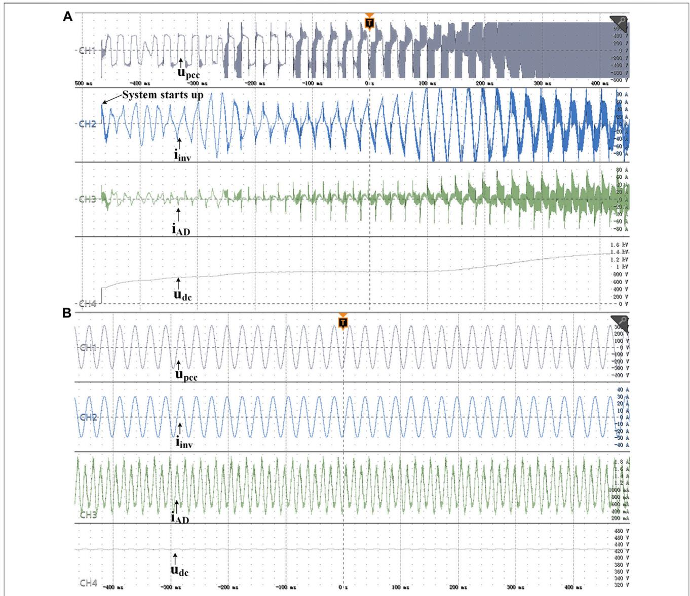
**FIGURE 13 |** Waveforms of grid-connected inverter system with active damper with different SOGI-PLL bandwidth  $f_{BW}$ . **(A)**  $f_{BW} = 1000$  Hz. **(B)**  $f_{BW} = 100$  Hz.
