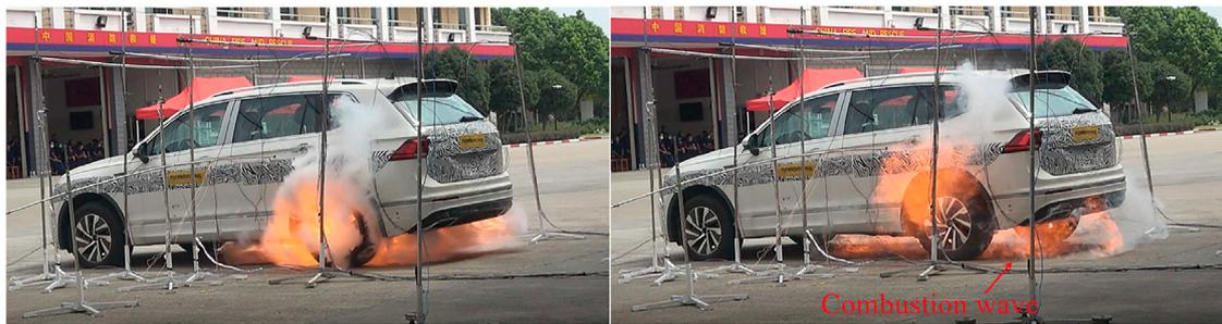
**FIGURE 3** | Explosion phenomenon in Test 1.
