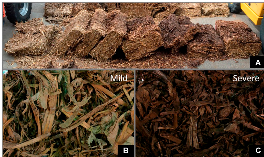
FIGURE 1 | (A) A dissected bale showing various degrees of biological degradation, (B) a closer look at the mildly degraded section showing little to no browning, and (C) severely degraded corn stover appearing very dark, nearly black (images provided by staff at Idaho National Laboratory*).
