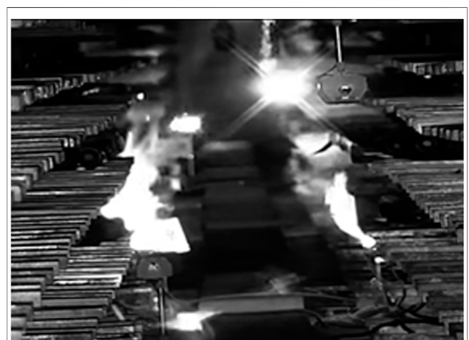
FIGURE 6 | Development of cable combustion in tunnel.
