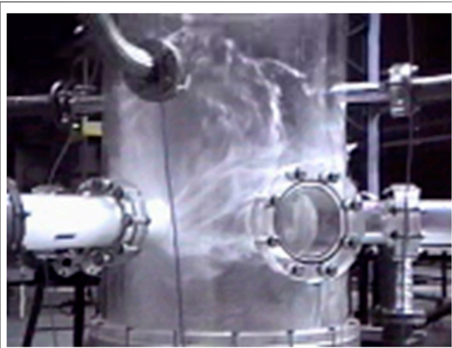
FIGURE 1 | ECC bypass phenomenon in RV downcomer (Cho et al., 2005).
