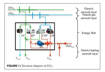
The ECU supports the multizone expansion, where the units are connected to each other through a power grid, natural gas network, and DHN, becoming the main body of the MRIES.
