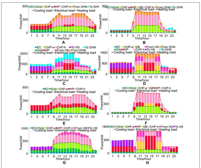
FIGURE 11 | Energy components of the EHs in scenario A and B. (A) Energy components of EH1 in scenario A. (B) Energy components of EH2 in scenario A. (C) Energy components of EH3 in scenario A. (D) Energy components of EH4 in scenario A. (E) Energy components of EH1 in scenario B. (F) Energy components of EH2 in scenario B. (G) Energy components of EH3 in scenario B. (H) Energy components of EH4 in scenario B.
