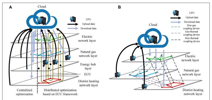
FIGURE 2 | Data flow of different optimization methods in IES. (A) Data flow of the centralized optimization and the ECU architecture distributed optimization. (B) Data flow of the distributed optimization decoupled according to energy networks.
