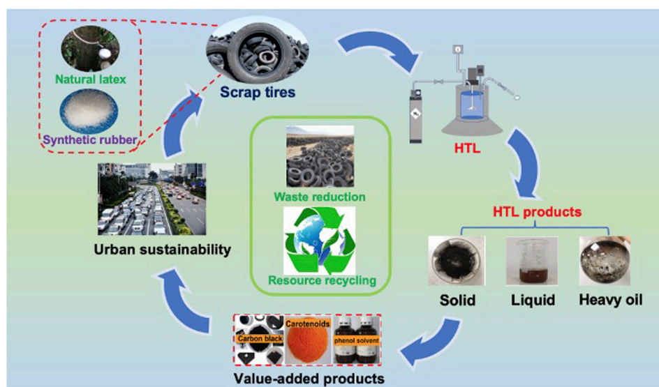
FIGURE 1 | Schematic diagram of the tire recycling process and concept through hydrothermal treatment.
