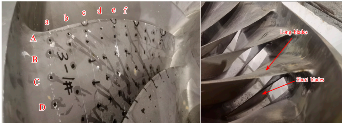
FIGURE 12 Measuring point of ultrasonic thickness gauge for turbine blades.
