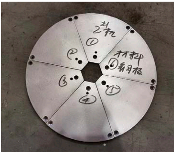
FIGURE 6 Wear test bench specimen.
