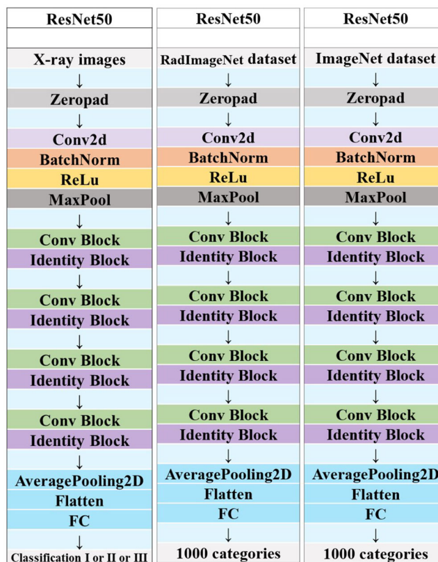
FIGURE 6 Schematic diagram of the deep convolutional neural network pre-training and fine-tuning network structure.
