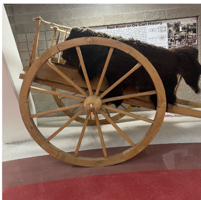
FIGURE 4 Red River cart images. (A) Red River Cart showing the dished wheel. (B) Red River Cart at center of TMC main building.
