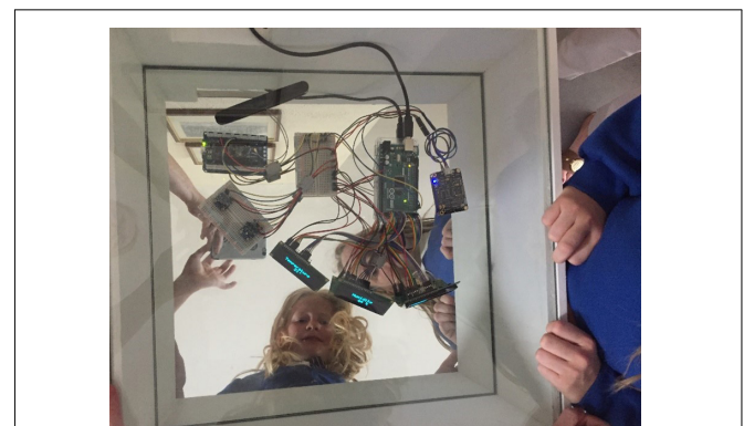
FIGURE 3 | Children looking into the Arduino boards which are connected to sensors, collecting data on light, humidity, temperature, and sound levels of the school environment (Morrin and Liston, 2020).
