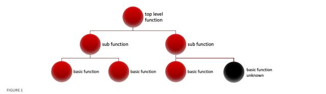
Reverse engineering is expressed schematically as performance of a functional analysis (Cummins, 1975, Cummins, 2000). The top level function of the whole system is decomposed into sub-functions, which can themselves be explained in terms of the interaction of basic functions. See also Bechtel and Richardson (2010) on the research strategy of functional decomposition, employed for investigating modular, hierarchical systems.
