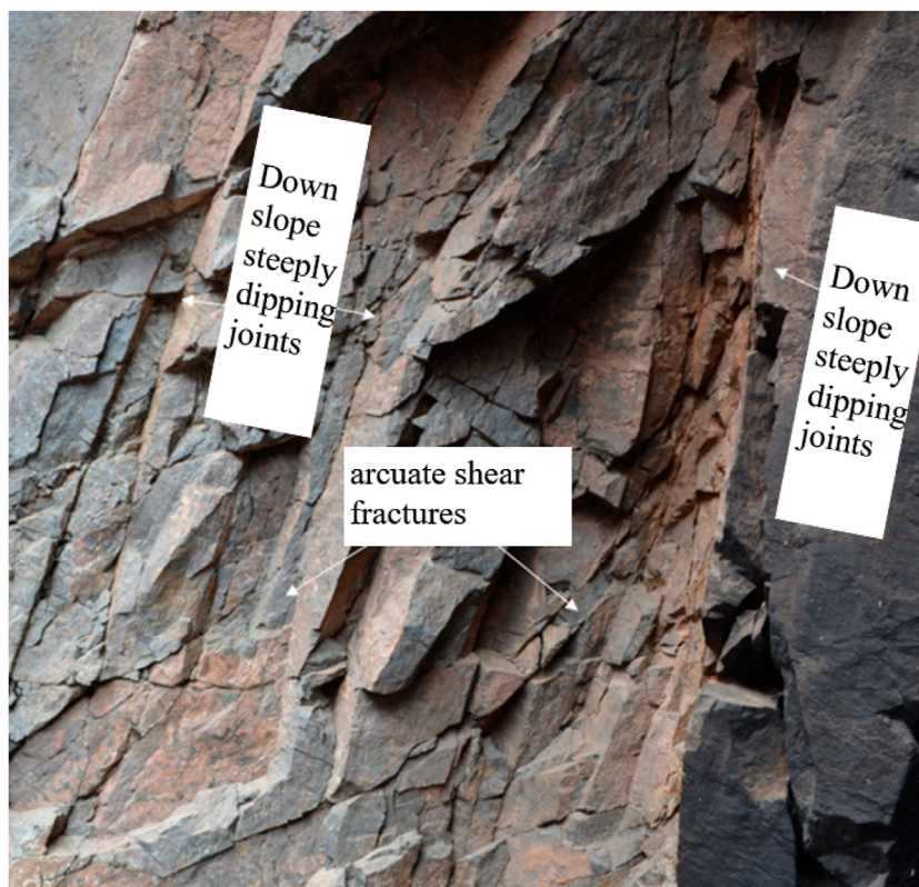
FIGURE 11 Rock mass fracture phenomenon at the tip out end of macroscopic joints on M bank slope.
