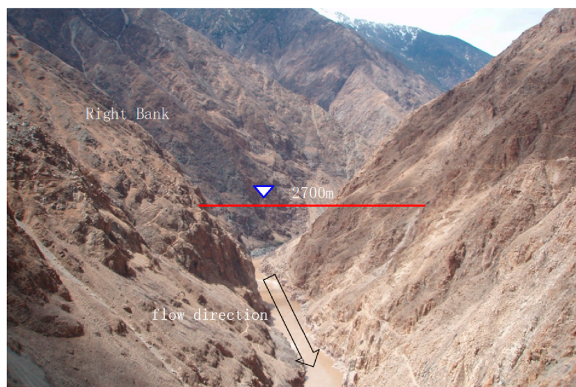
FIGURE 5 Morphology of the valley bank slope in the M section of the Lancang River.
