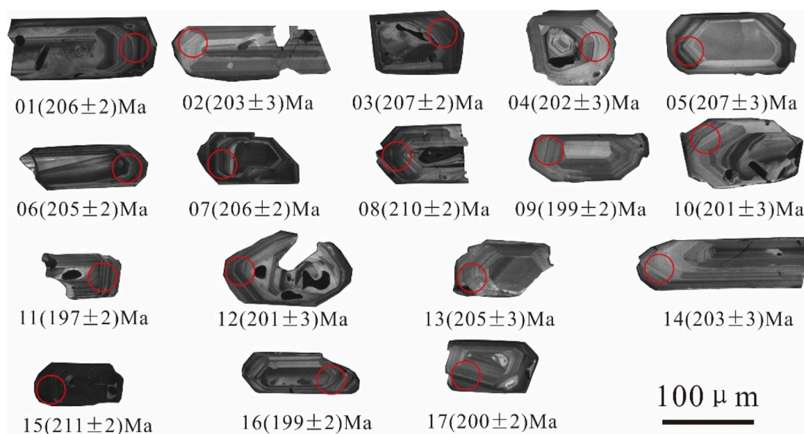
FIGURE 8 Cathodoluminescence (CL) image of zircons from the syenogranite in the Xiaohulin lead-zinc mining area.
