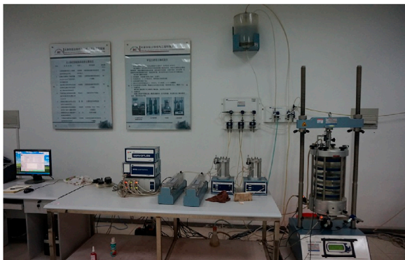
FIGURE 3 Wykeam Farrance stress path triaxial instrument used in this work.
