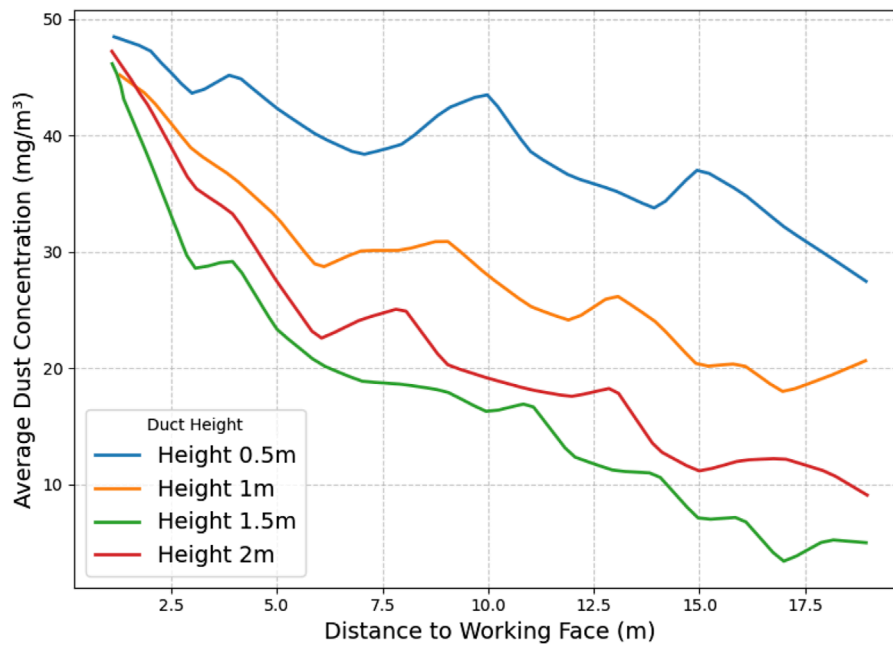
FIGURE 12 Average dust concentration distribution across the roadway cross-section for different duct heights.
