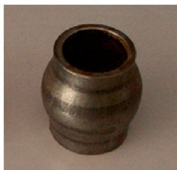
FIGURE 2 Spherical yielding tube and its deformation after compression.
