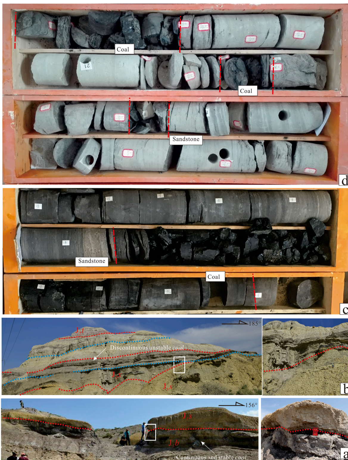
FIGURE 4 Coal of distribution with coal-bearing strata of Middle-Lower Jurassic in Hongshanzui area in the Junggar Basin. (A) Continuous and stable coal seams, developed in J_{1b1} , located in northwestern margin of the Junggar Basin; (B) discontinuous and unstable coal seams, developed in J_{2x2} , located in northwestern margin of the Junggar Basin; (C) continuous and stable coal seams of the J_{1b1} observed in the core; and (D) discontinuous and stable coal seams of the J_{2x2} observed in the core.
