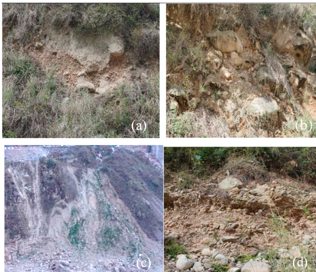
FIGURE 5 Overburden on the left bank of Badi Township. (A) The alluvial-diluvial strata exposed above; (B) The alluvial layer exposed at the edge of the highway; (C) The artificial accumulation next to the highway before water storage; (D) The alluvial sand and gravel along the riverbank before water storage.
