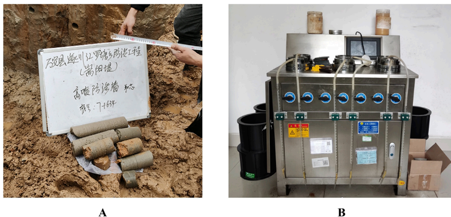
FIGURE 9 Core drilling and permeability coefficient testing equipment. (A) Core drilled samples. (B) SS-2.5 Penetrometer.
