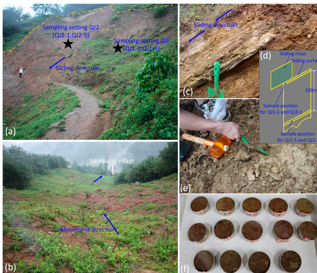
FIGURE 2 Overview of the sliding source area and soil sampling locations: (A,B) Sliding source area showing sampling sites and landslide flow zone. (C-E) Photographs and schematic illustrations of the sampling. (F) Soil samples prepared for laboratory testing.
