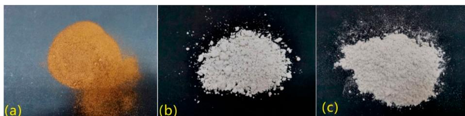
FIGURE 2 Chemical stabilisers (A) Calcium Lignosulphonate (LS); (B) Lignin Fibre (LF); (C) Lime (LI).
