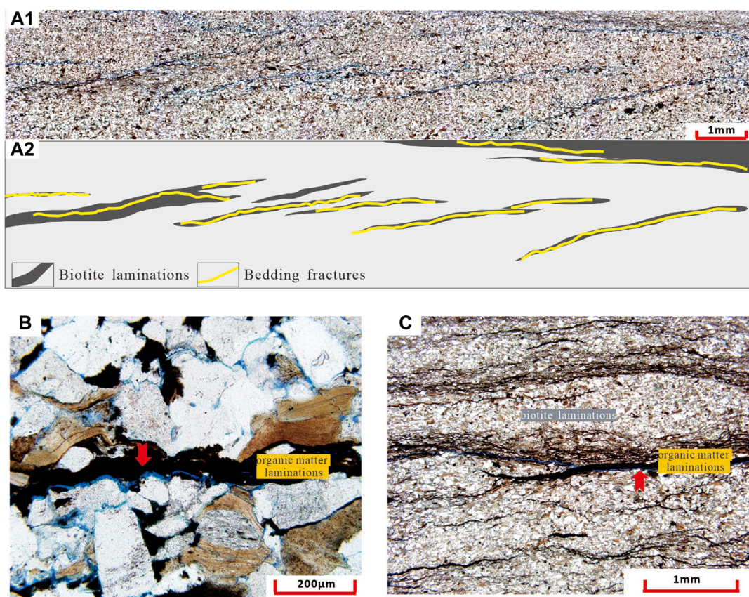
FIGURE 5 Morphological characteristics of bedding-parallel fractures in tight sandstone of the Chang 7 reservoir in the Ordos Basin. (A1) BPFs develop along the biotite laminations, with unfilled fractures marked in blue (Well W1,1999.5 m, plane-polarized thin sections), (A2) a sketch of (A1) , the biotite laminations in black and the BPFs in yellow. (B) BPFs develop along the edges of organic matter laminations, with unfilled fractures shown in blue (Well B1,1960.1 m, plane-polarized thin sections). (C) BPFs develop along the boundaries of biotite and organic matter laminations, where the laminations pinch out and the BPFs terminate. (Well W1,2005.4 m, plane-polarized thin sections). Red arrows indicate BPFs.
