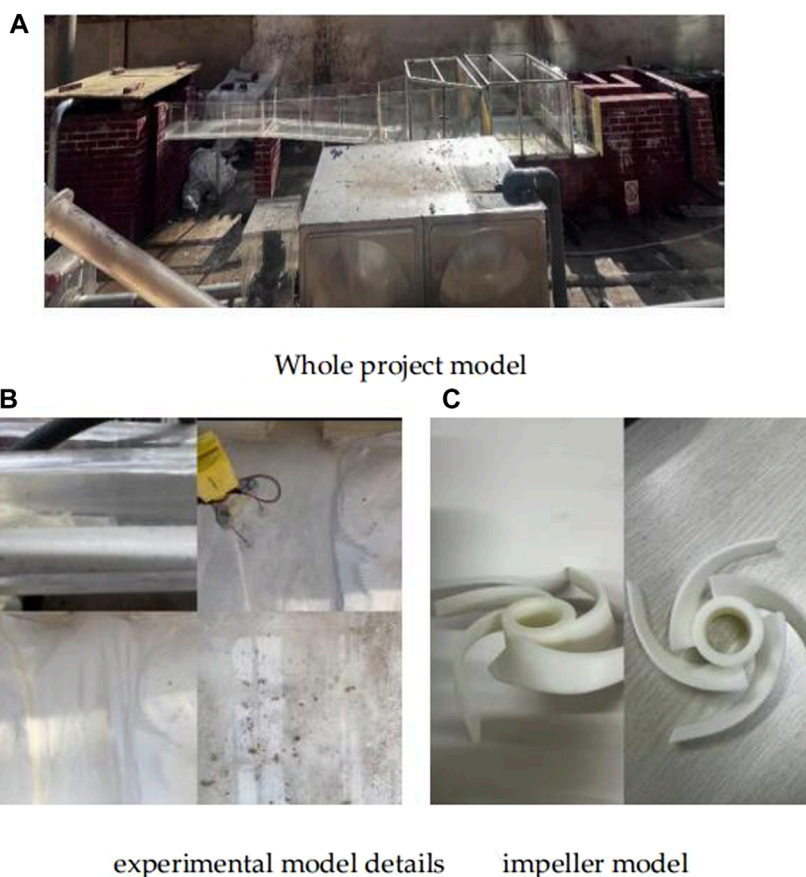
FIGURE 8 Experimental model. (A) Whole project model. (B) experimental model details. (C) impeller model.
