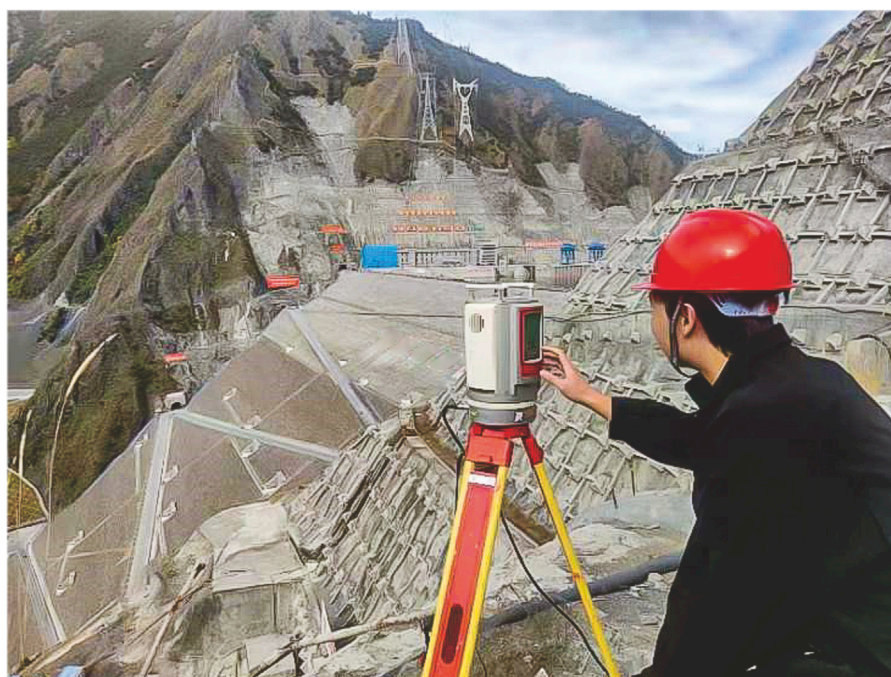
FIGURE 3 On-site data acquisition using a Riegl-VZ 2000i.
