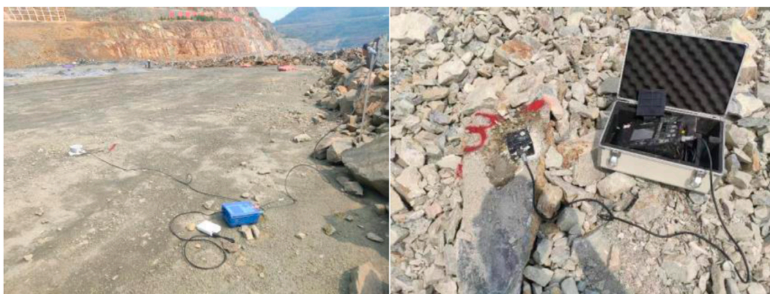
FIGURE 4 Placement of site monitoring points.
