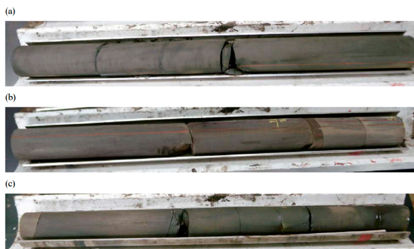
FIGURE 3 Hydraulic fracture doublets in three tubes from Core 3: (A) in the middle of the tube, (B) above the yellow foot marker, (C) center left of the tube. (Gale et al., 2021) (The diameter of the core in the figure is 3 in).
