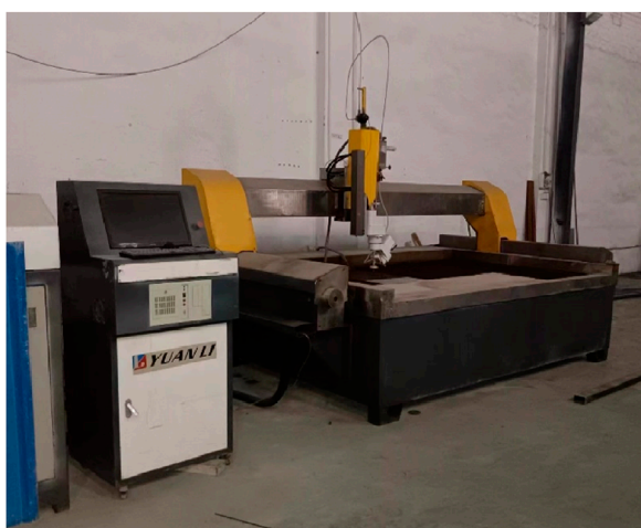
FIGURE 4 Preparation of rock specimen cracks by cutting.
