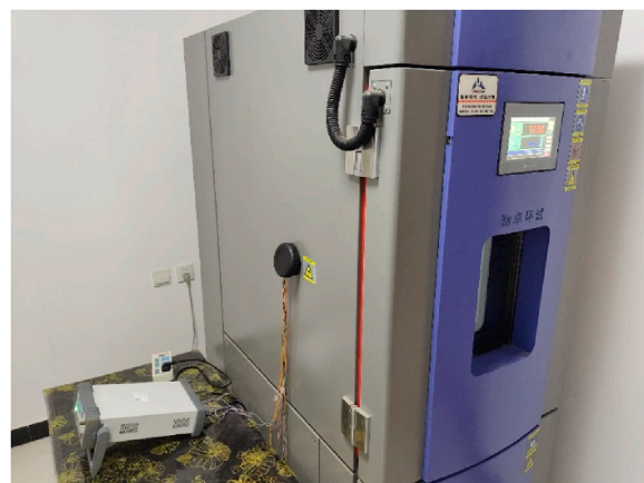
FIGURE 5 Freeze-thaw strength testing machine.
