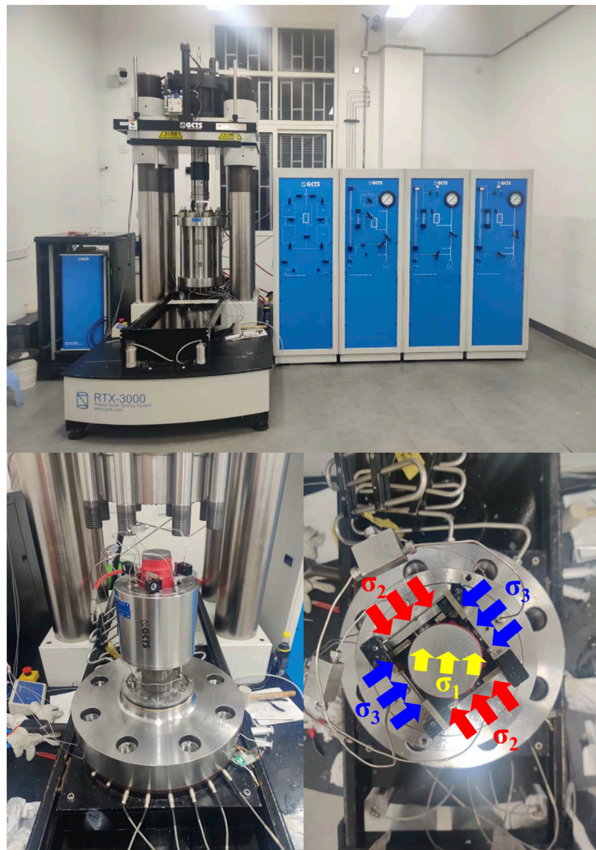
FIGURE 2 RTX-3000 experimental system of high-temperature and high-stress rock mechanics. Note that the yellow, red, and blue arrows represent the loading directions of the three principal stresses of \sigma_1 , \sigma_2 , and \sigma_3 during the true triaxial flow experiments.
