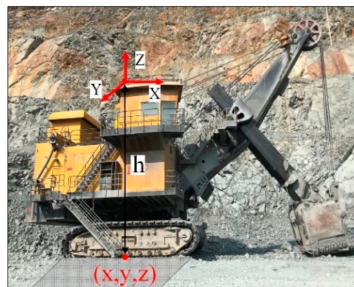
FIGURE 1 Position measurement during movement of the electric shovel.
