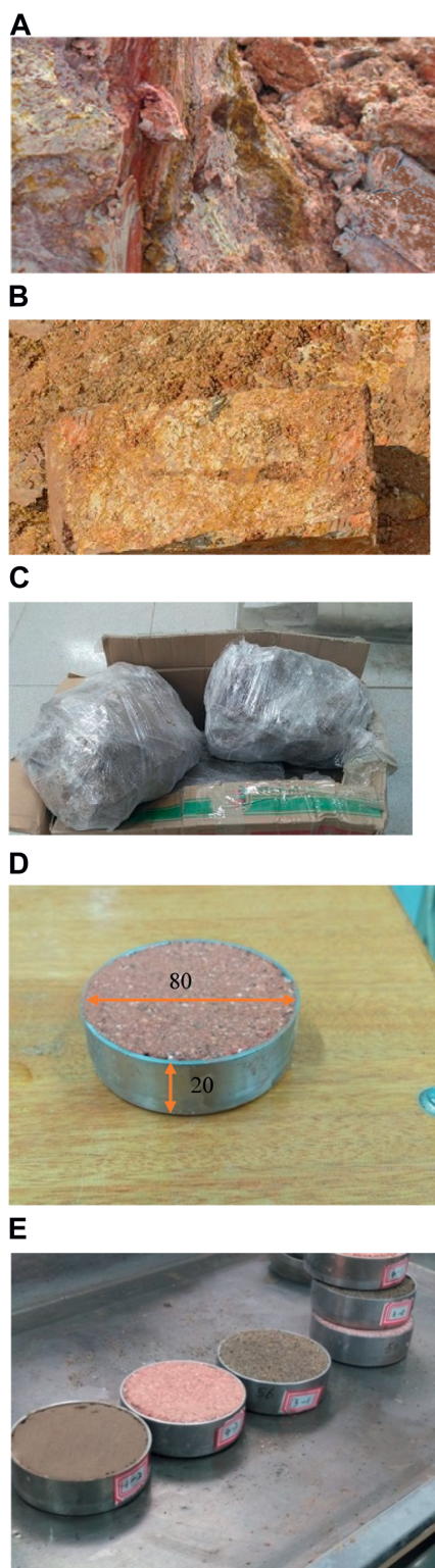
FIGURE 2 Sampling on site and the production of soil sample specimens. (A) The site of soil sampling; (B) A soil sample obtained on site; (C) The packaging of soil samples; (D) The dimensions of a soil sample specimen; (E) Multiple soil sample specimens.
