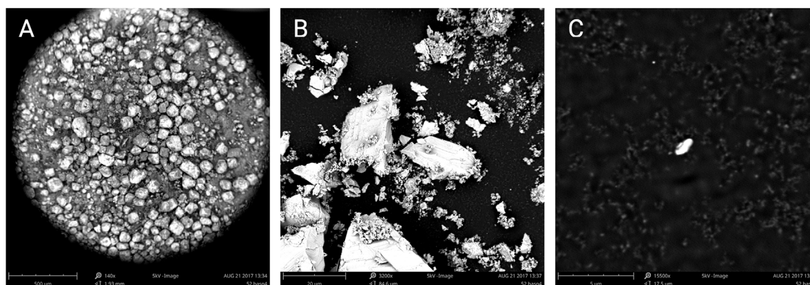
FIGURE 4 Scanning electron microscope images of the barite-containing fraction of GOA sediment. (A) Overview of the remaining sample at a 500 µm scale. (B) A portion of the remaining sample at a 20 µm scale. (C) A highly refractory mineral, possibly barite, at a 5 µm scale.
