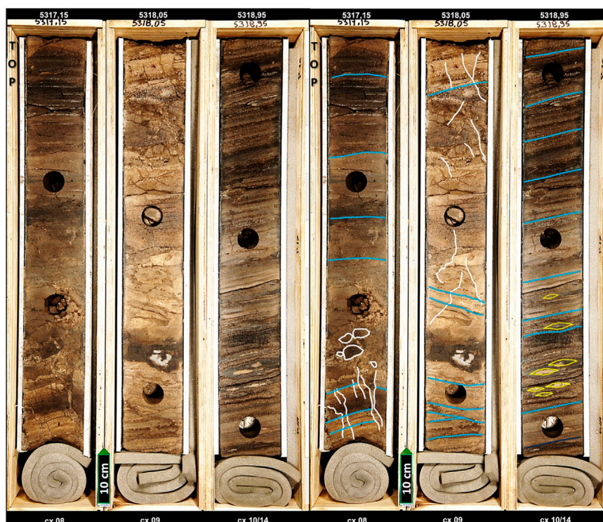
FIGURE 11 Core photograph from well the 3-BRSA-967A-RJS (after Costa et al., 2017), showing representative lithologies of travertine-like carbonates: wackestones containing in situ and reworked shrubs and spherulitic grainstone levels locally varying for micro-conglomerates, silicified breccias, vuggy porosity among the shrubs, and fracture zones.
