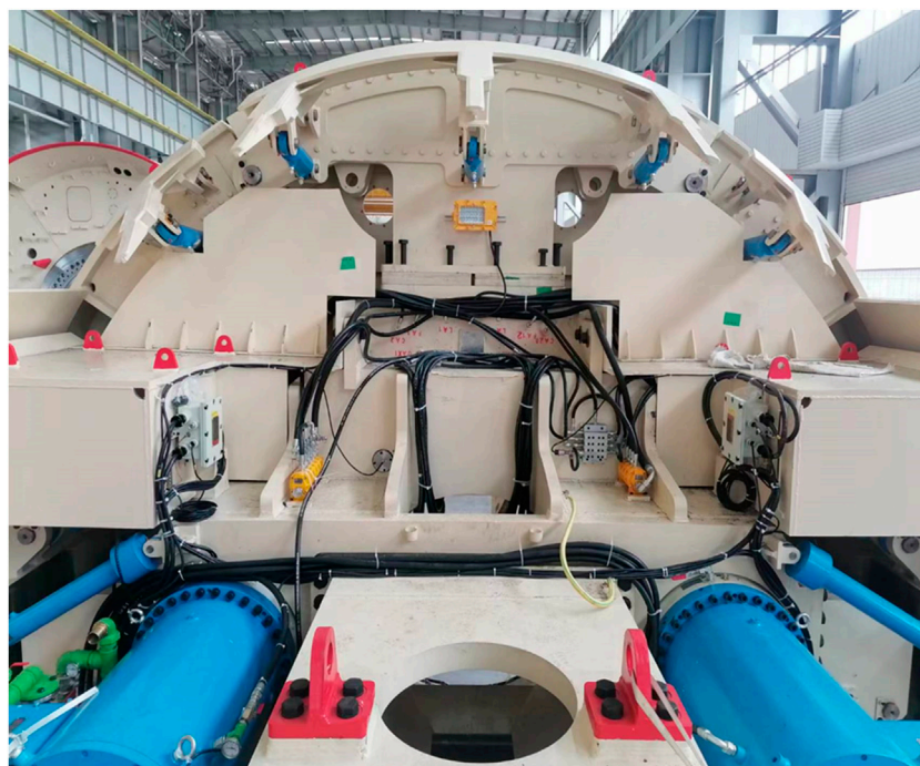
FIGURE 11 Main beam reserved for the slag collecting port.
