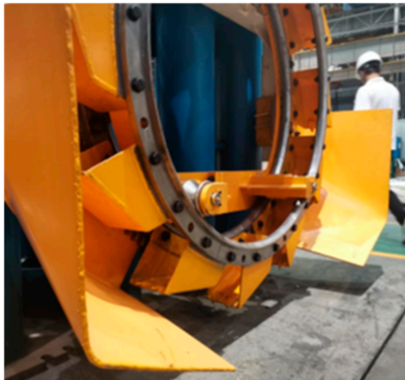
FIGURE 9 Slag cleaning bucket wheel machine.
