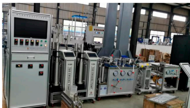
1-High pressure compressor, 2-Piston container, 3-Constant speed constant pressure pump, 4-Pressure gauge, 5-Manual pressure regulating valve, 6-Back pressure system, 7-Preheater, 8-Safety valve, 9-Positive and negative drive controller, 10-Core holder, 11-Sand collecting container, 12-Electronic balance
