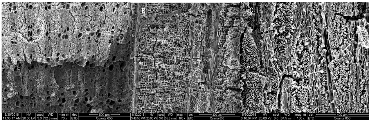
FIGURE 7 SEM microphotographs of Tamarix . (A) TS; (B) RLS; and (C) TLS.
