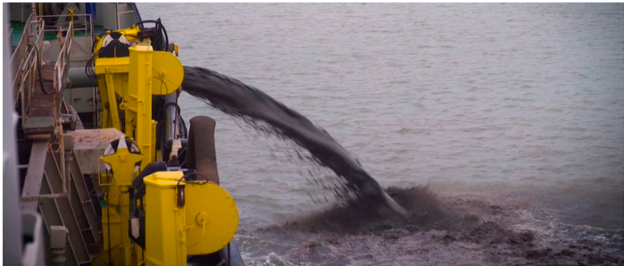
FIGURE 3 Water column recharge by TSHD.
