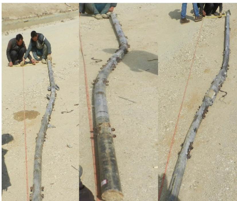
FIGURE 14 Steel flower tube failure of the second, third, and fourth group experiments.
