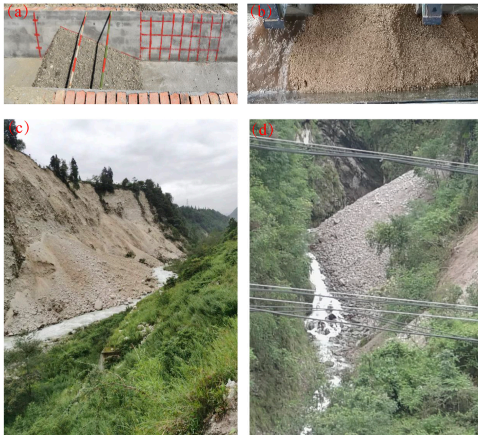
FIGURE 3 Comparison of experimental landslide dams and prototypes: (A) manual stacked dam; (B) natural sliding dam in this paper; (C,D) are photographs of landslides blocking river.
