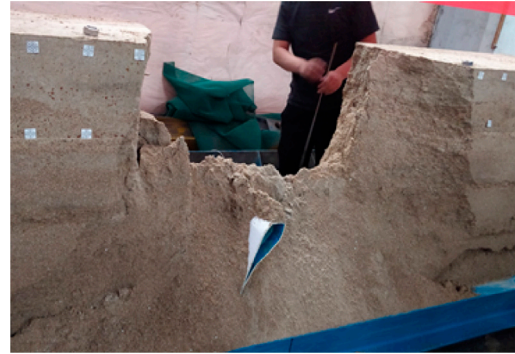
FIGURE 4 | Real picture of tunnel collapse and even surface collapse.
