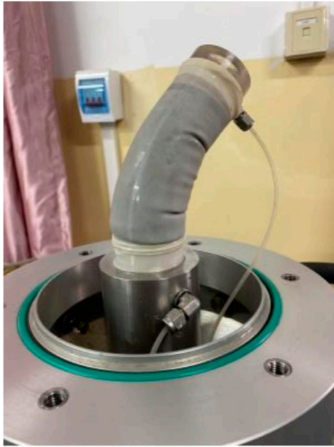
FIGURE 10 | Softening phenomenon of PG after liquefaction by bidirectional vibrations.
