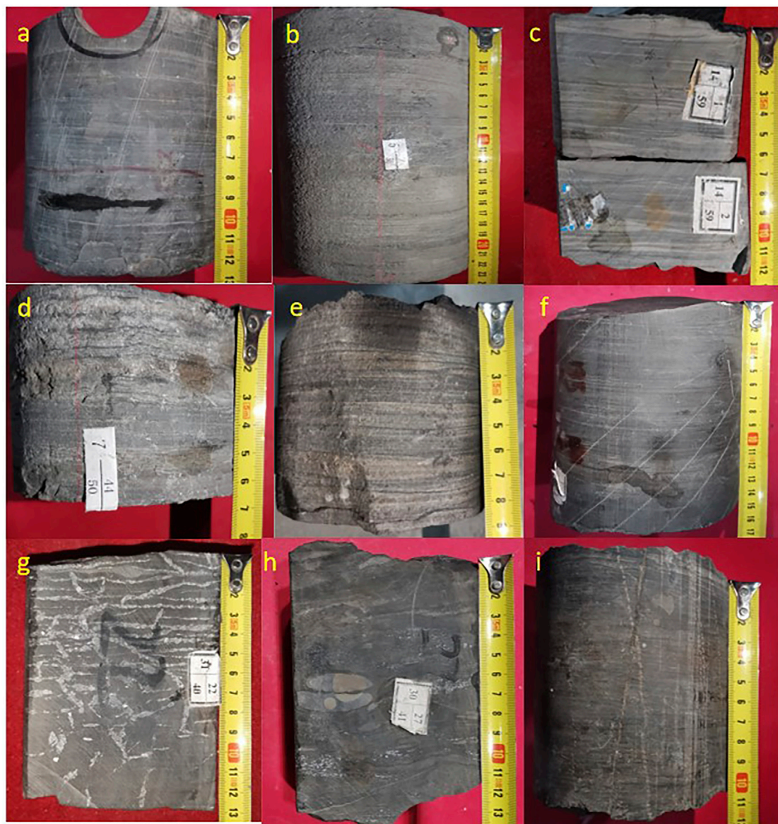
FIGURE 2 | Core of Six Types of Rocks in the Lucaogou Formation of the Jimsar Sag. (A) 33/38 1st Barrel No. J251 Well, dark grey calcareous mudstone; (B) 26/50 5th Barrel No. J10024 Well, dark grey argillaceous dolomite; (C) 1, 2/59 14th Barrel No. J10025 Well, light grey argillaceous dolomite; (D) 44/50 7th Barrel No. J10024 Well, dark grey marlite; (E) 58/70 1st Barrel No. J32 Well, light grey dolomitic siltstone; (F) 15/35 5th Barrel No. J305 Well, grey black dolomite mudstone; (G) 22/40 31st Barrel No. J10025 Well, grey black argillaceous siltstone; (H) 27/41 30th Barrel No. J10025, dark grey calcareous siltstone; (I) 63/74 5th Barrel No. J251 Well, dark grey silty mudstone.
