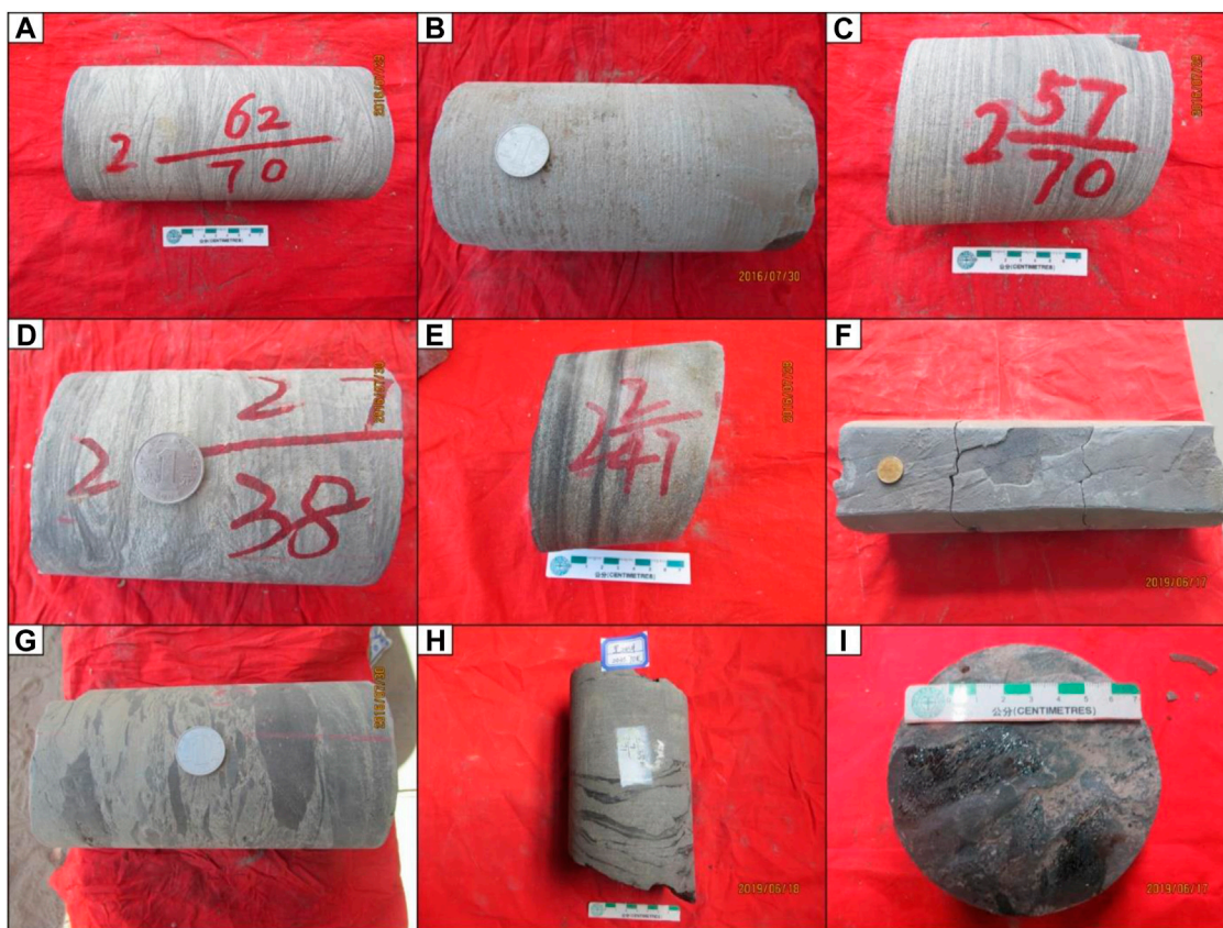
FIGURE 3 | Core photos of Yangchang formation in study area. (A) Cross bedding; (B) Massive bedding; (C) Parallel bedding; (D) Convoluted bedding; (E) Oblique bedding; (F) Fractures; (G) Mud gravel; (H) Muddy strip; (I) Scratch.
